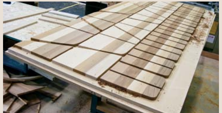
Parts for the 2010 Olympic medal ceremonies podiums in the CAWP lab after CNC machining.
