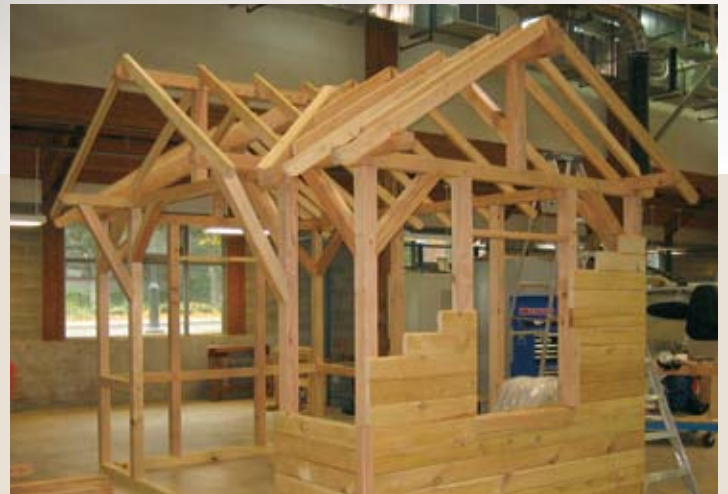
Product development: A timber-frame gazebo prototype cut on the Hundegger K2.
