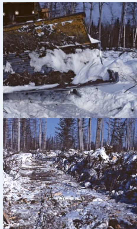
Figure 2 A & B. Crawler tractor with a Rome KG blade used for stump shearing. An in-block winter access road built using stump shearing.
