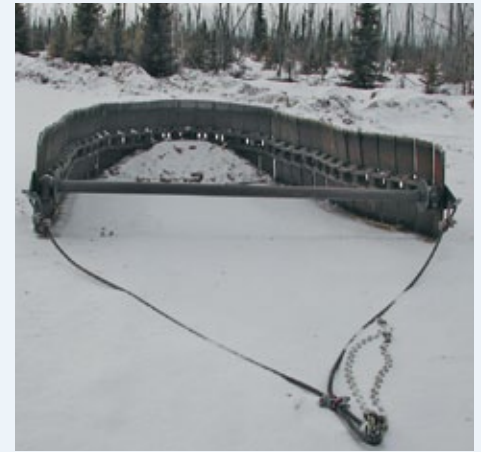
Figure 4. Drag equipment used along winter roads includes used excavator tracks and skidder tires.
